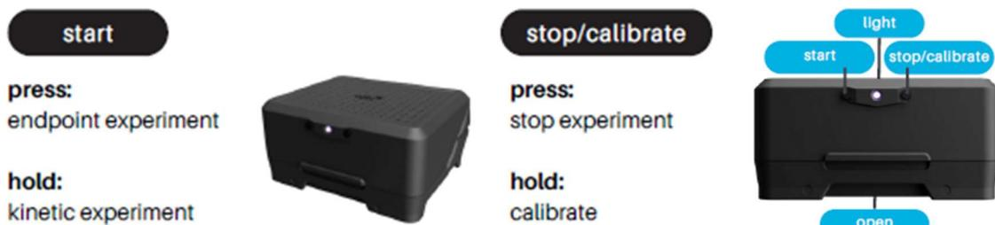
The “start” (left) button has two functions. Start an endpoint read by *pressing and quickly releasing* the “start” button. To start a kinetic read, *press and hold* the “start” button until the status light (center) flashes white. At this point, the Rayo S600 will perform an automatic calibration to the plate and sample (cyan light) and then automatically begin readings at the designated time intervals (default five minutes; green light).
