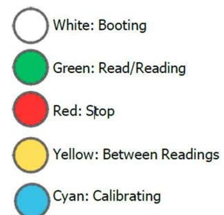
The “stop/calibrate” button also has two functions. If *pressed and quickly released*, the Rayo S600 will complete the experiment and halt measurements (red light). For samples at high OD and/or high shaking RPM, the Rayo S600 may take up to 2 seconds to stop after pressing. If *pressed and held* when an experiment is not running, the Rayo S600 will perform a device calibration (cyan light).
